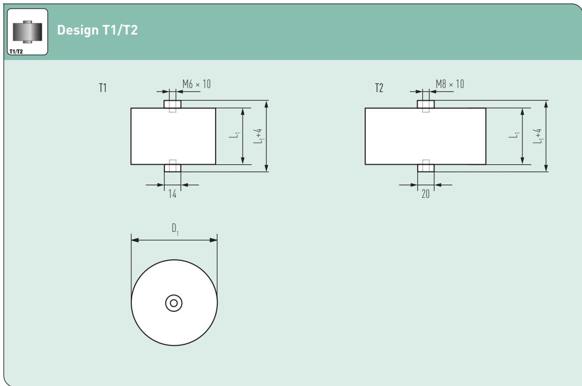
**T1 CAPACITORS WITH A CAN DIAMETER OF 55...60 mm****T2 CAPACITORS WITH A CAN DIAMETER OF 75...115 mm**
