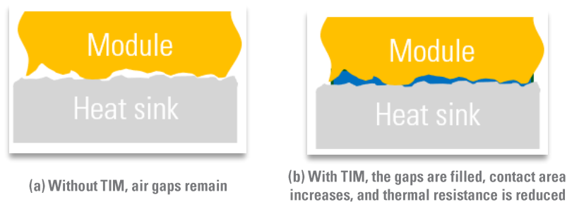
Figure 5. Improving Thermal Transfer by using Thermal Interface Material (TIM)
