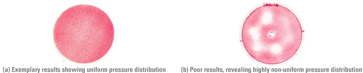
Figure 12. Results from Inspecting Pressure Distribution Using Color-Changing Film
