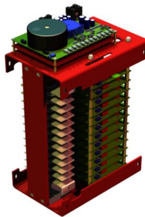
Figure 1: Example of a Stacked Arrangement of High-power Semiconductors
