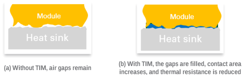
Figure 5. Improving Thermal Transfer by using Thermal Interface Material (TIM)
