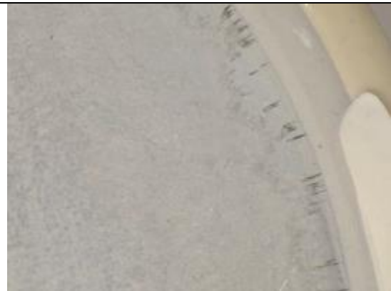
Figure 2: Initial evidence of thermal cycling scrubbing at the edge on the cathode contact area
