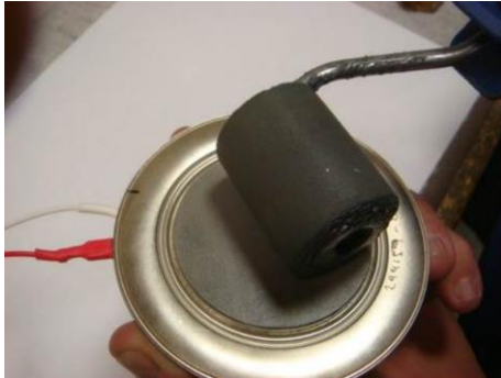
(a) Applying a very small amount of contact grease with a roller
