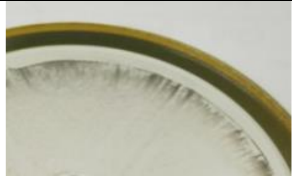
Figure 4: More extensive evidence of thermal cycling scrubbing at the edge on the cathode contact area
