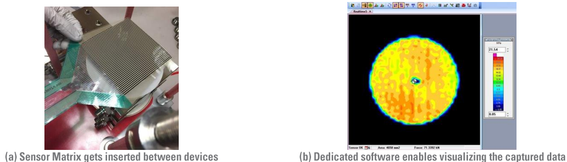
Figure 13. Piezo-electric, Tactile Pressure Sensor, and Captured Results
