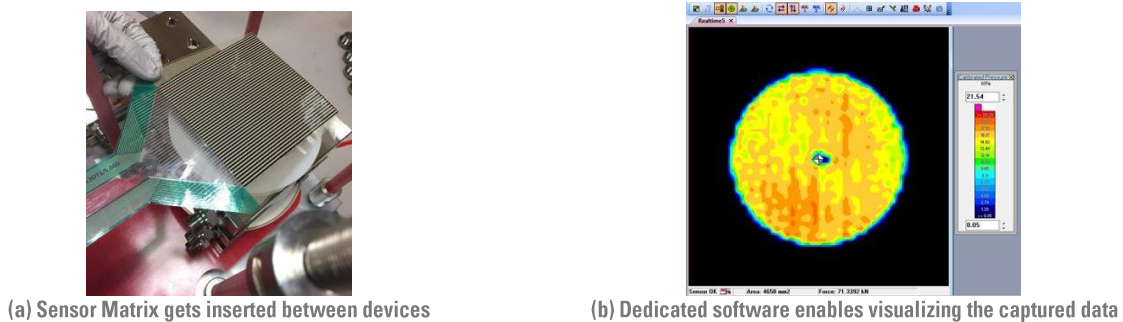
Figure 13. Piezo-electric, Tactile Pressure Sensor, and Captured Results
