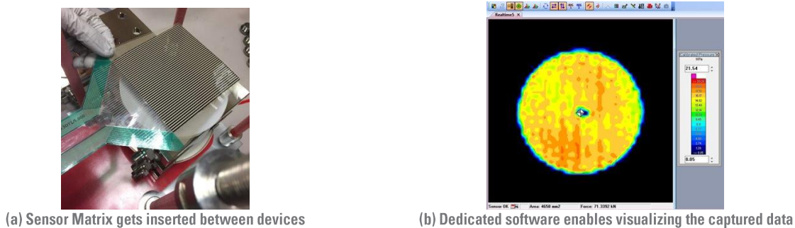
Figure 13. Piezo-electric, Tactile Pressure Sensor, and Captured Results
