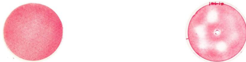
(a) Exemplary results showing uniform pressure distribution (b) Poor results, revealing highly non-uniform pressure distribution
