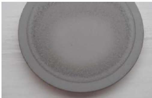
Figure 3: Initial evidence of thermal cycling scrubbing on the anode molybdenum contact
