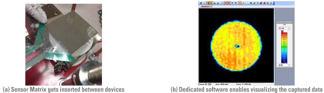
Figure 13. Piezo-electric, Tactile Pressure Sensor, and Captured Results
