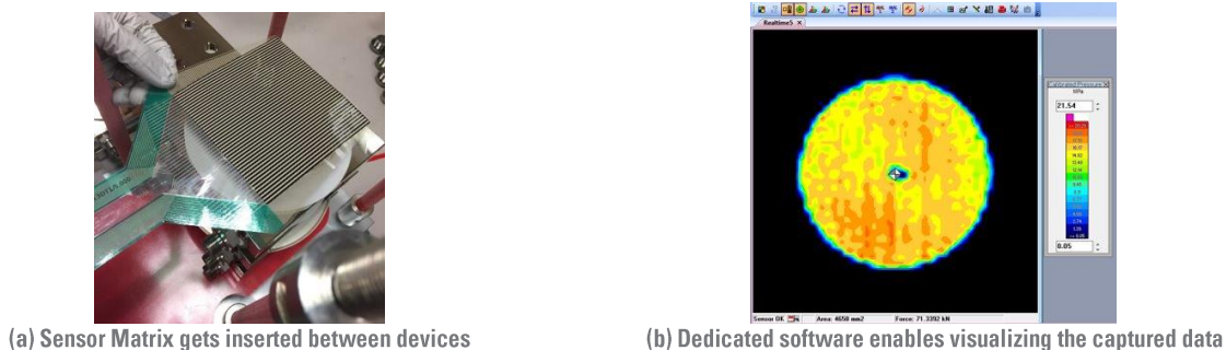
Figure 13. Piezo-electric, Tactile Pressure Sensor, and Captured Results
