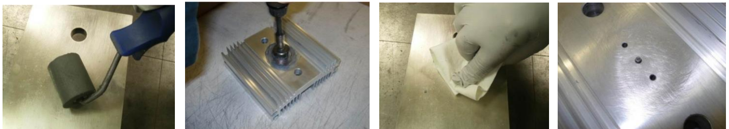
(a) Contact grease is applied to the surface sparingly (b) Abrasion of the heatsink using contact grease and rotating wire brush (c) Cleaning the surface right before mounting the disc (d) Mounting surface, lightly abraded
