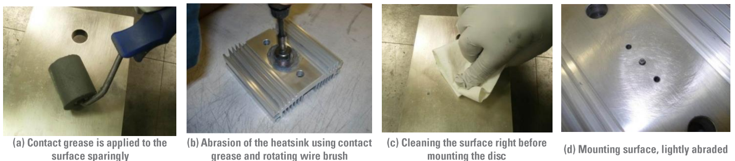
Figure 5. Surface Preparation Sequence
