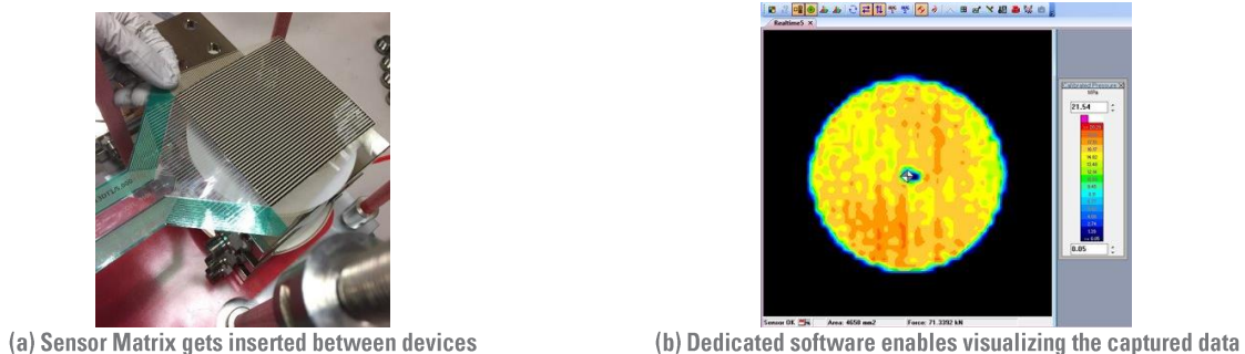
Figure 13. Piezo-electric, Tactile Pressure Sensor, and Captured Results
