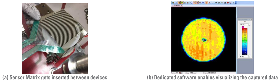
Figure 13. Piezo-electric, Tactile Pressure Sensor, and Captured Results
